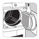
The filter in the inner door may be removed for cleaning. Do not be alarmed by the amount of fluff. It is not due to excessive wear caused by the dryer. All fabric loses fluff when drying but it goes un-noticed in the air. In a tumble dryer it simply collects in the filter. After a while, a withish patina due to detergent residue on laundry forms on the filters.
